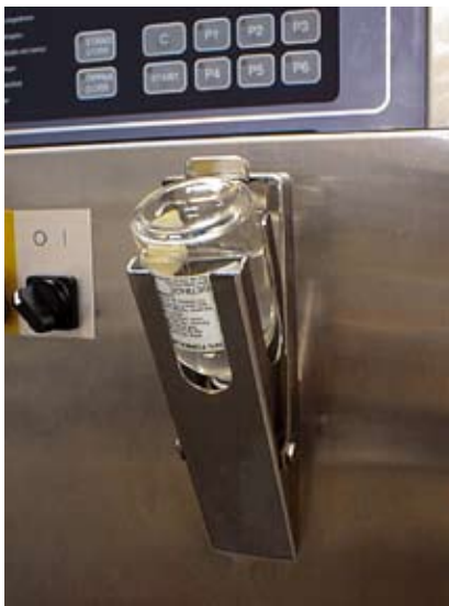
The Getinge HS66 LTSF sterilizer has an injection bottle holder for the formalin on front. The content inside the bottle can be easily observed before use. Alarm is activated when an empty bottle is used.
